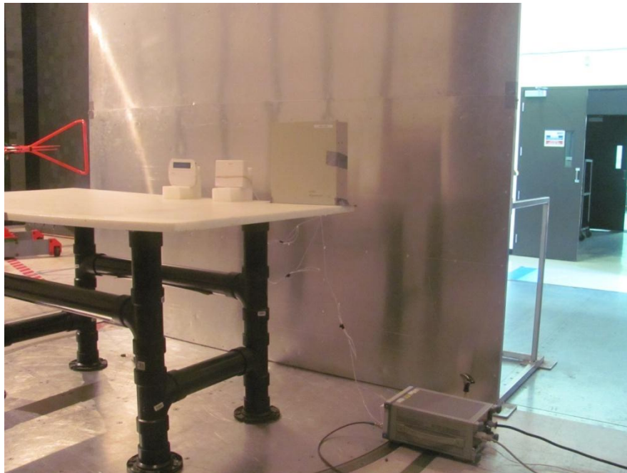
Photo 8.1-1: Conducted emissions setup
