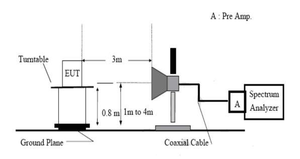
(C) Substituted Method Test setup:
