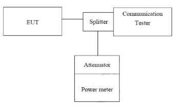
Measurement Setup for testing on Antenna connector.
