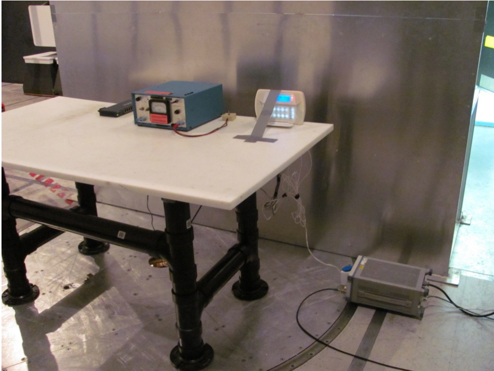
Photo 3: AC Conducted emissions setup
