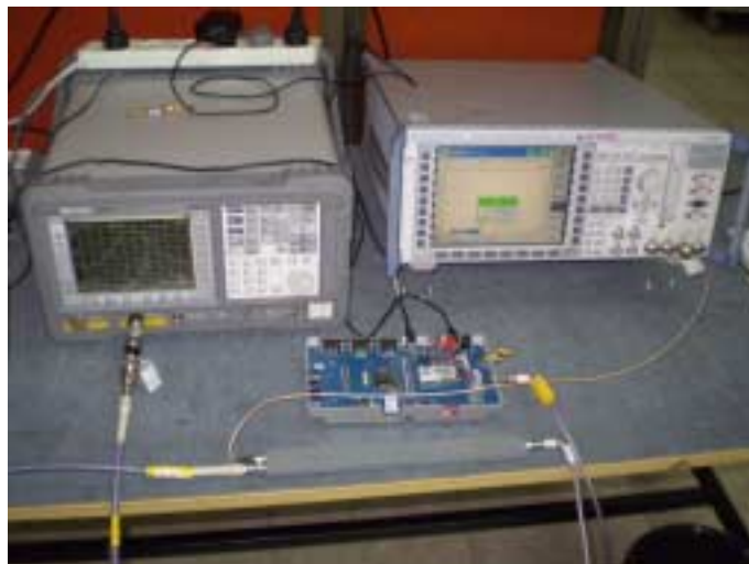
Photograph 8.3.1 Spurious emission test setup
