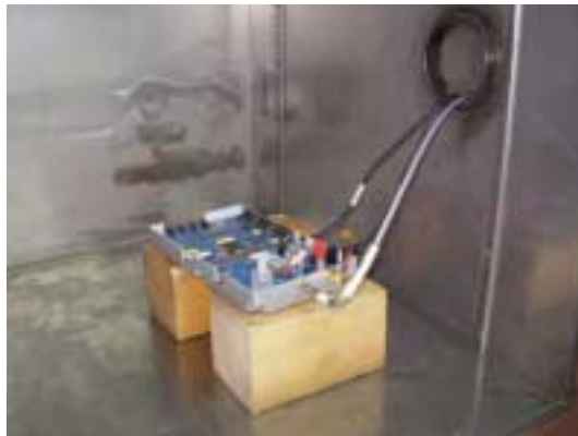
Photograph 8.5.2 Frequency stability test setup
