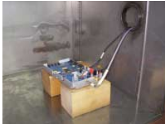
Photograph 7.5.2 Frequency stability test setup
