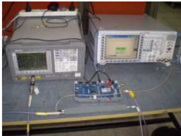
Photograph 7.2.2 Occupied bandwidth test setup
