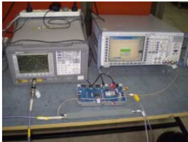
Photograph 7.3.2 Spurious emission test setup
