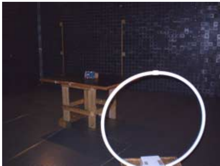
Photograph 8.4.1 Setup for spurious emission field strength measurements in 9 kHz to 30 MHz band
