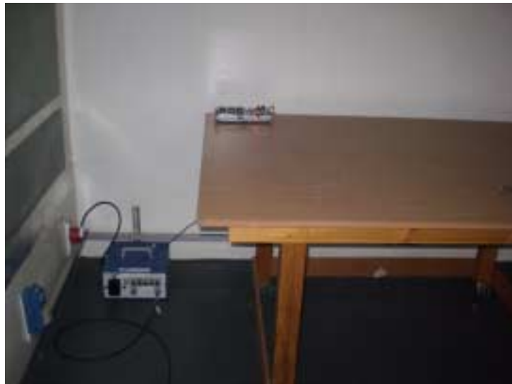
Photograph 9.1.1 Setup for conducted emission measurements
