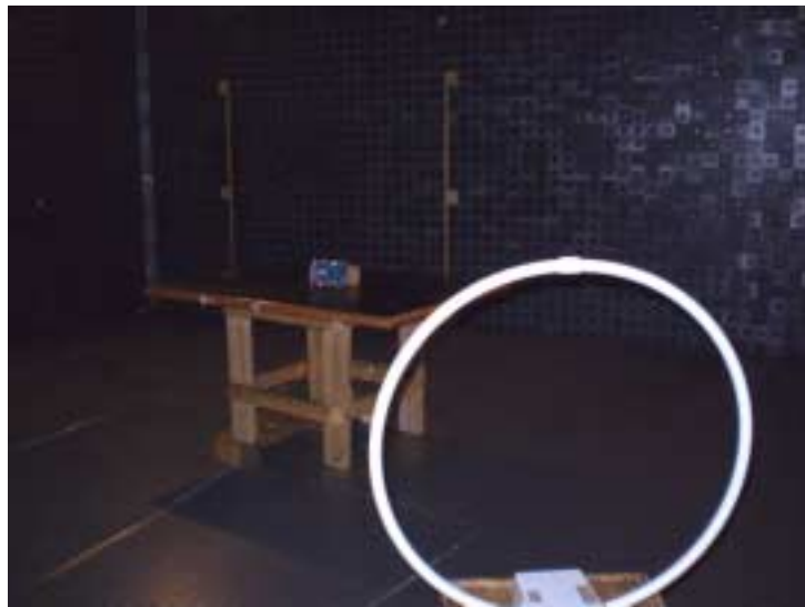
Photograph 7.4.1 Setup for spurious emission field strength measurements in 9 kHz to 30 MHz band
