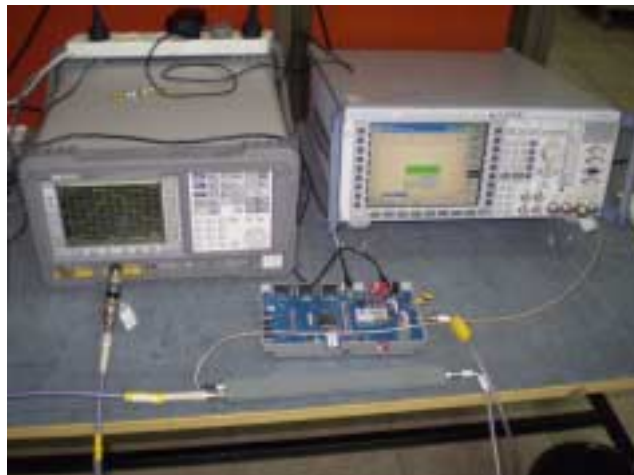
Photograph 8.1.1 Peak output power test setup
