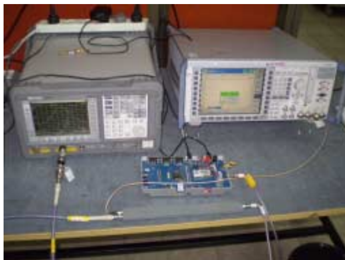
Photograph 9.3.1 Spurious emission test setup
