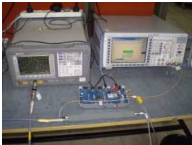
Photograph 7.1.2 Peak output power test setup
