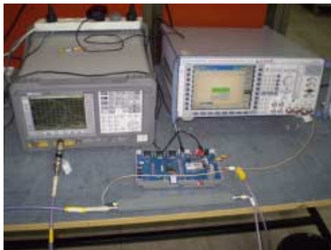
Photograph 8.2.2 Occupied bandwidth test setup
