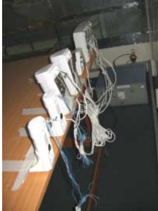
Photograph No.9 Setup for conducted emission measurements on the AC power lines
