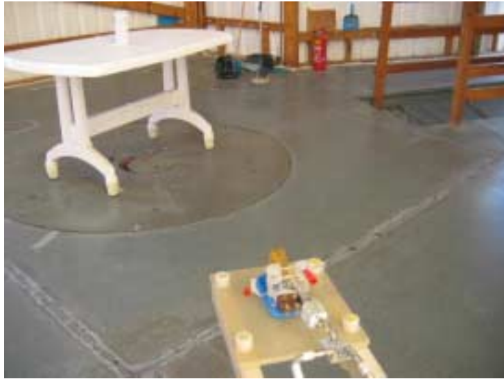
Photograph No.6 Setup for radiated emission measurements at the OATS above 40 GHz
