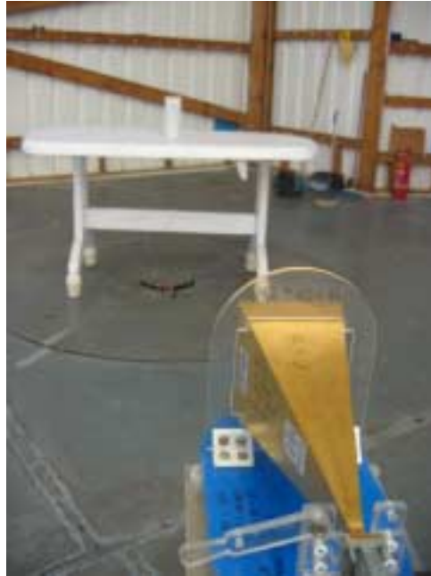
Photograph No.4 Setup for radiated emission measurements at the OATS from 18 to 26.5 GHz
