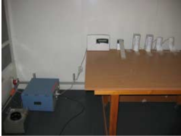
Photograph No.8 Setup for conducted emission measurements on the AC power lines
