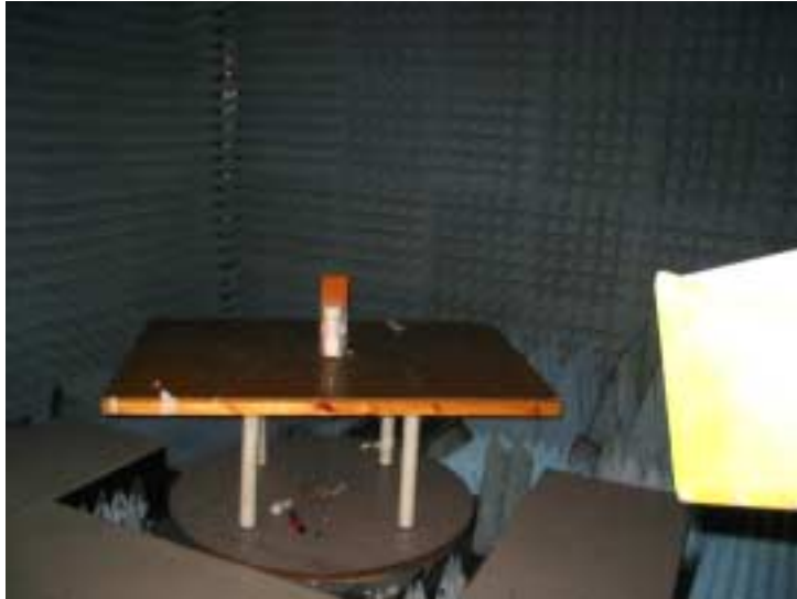
Photograph No.3 Setup for radiated emission measurements in the anechoic chamber from 1 to 18 GHz
