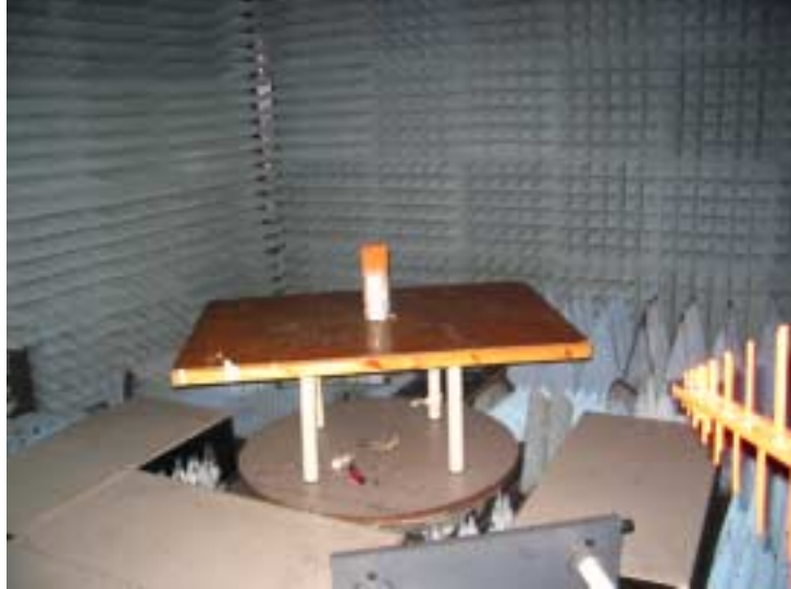
Photograph No.2 Setup for spurious emission field strength measurements in the anechoic chamber in 30 MHz – 1000 MHz range
