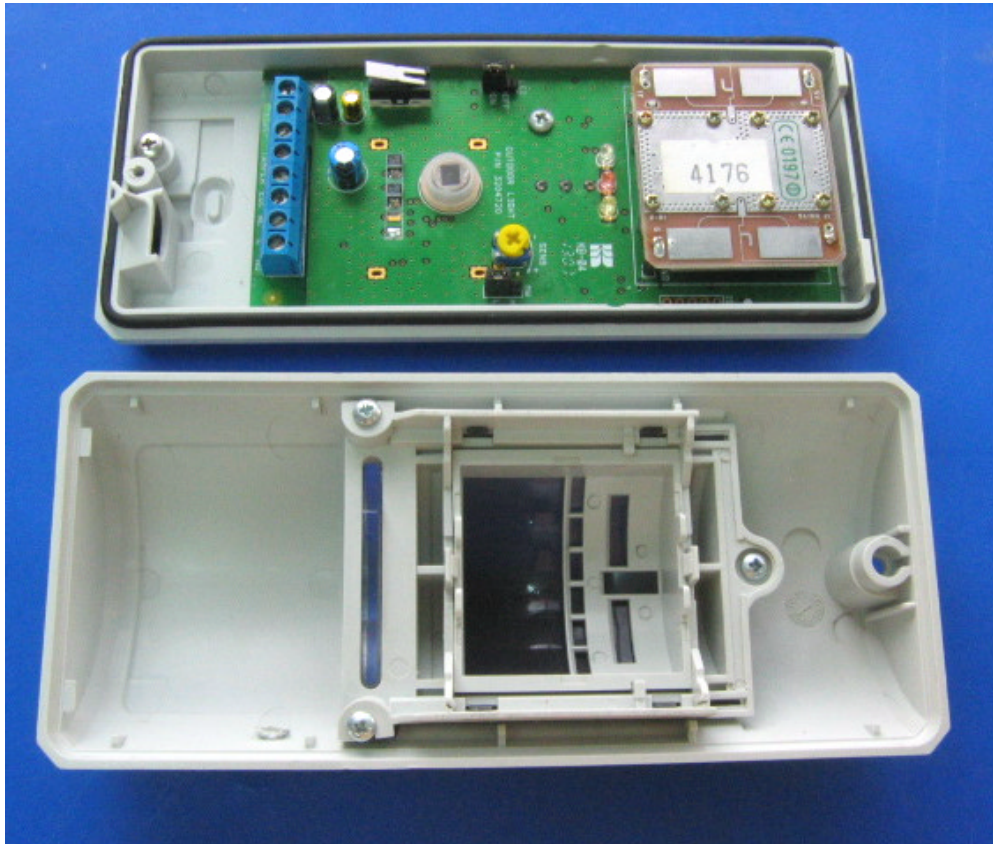
Photograph No.1 Detector internal view with removed front cover
