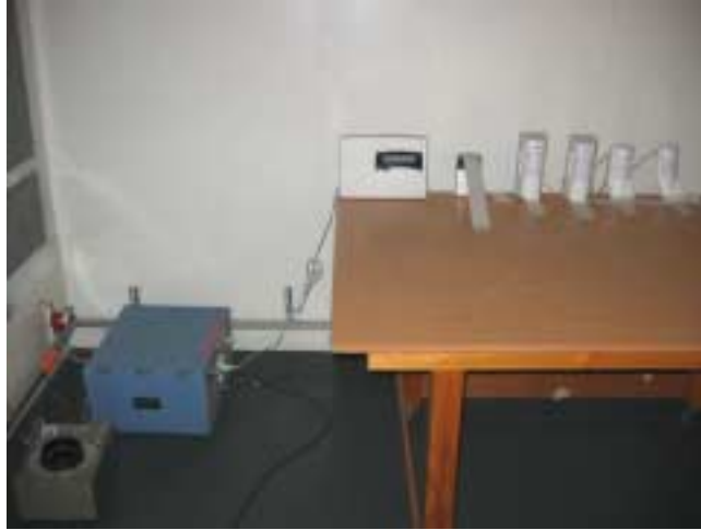
Photograph No.7 Setup for conducted emission measurements on the AC power lines
