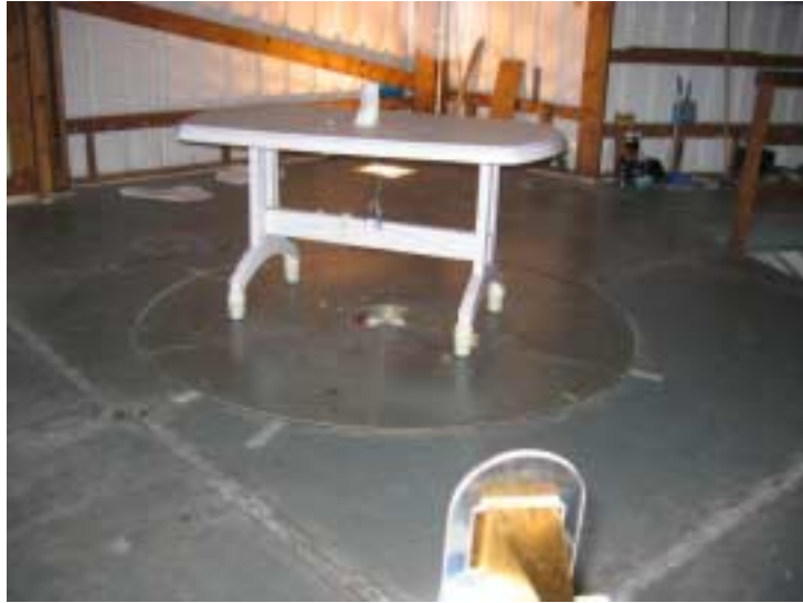
Photograph No.5 Setup for radiated emission measurements at the OATS from 26.5 to 40 GHz
