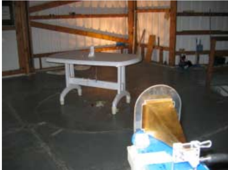
Photograph No.4 Setup for radiated emission measurements at the OATS from 18 to 26.5 GHz
