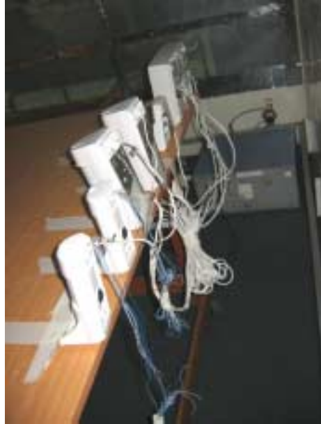
Photograph No.8 Setup for conducted emission measurements on the AC power lines
