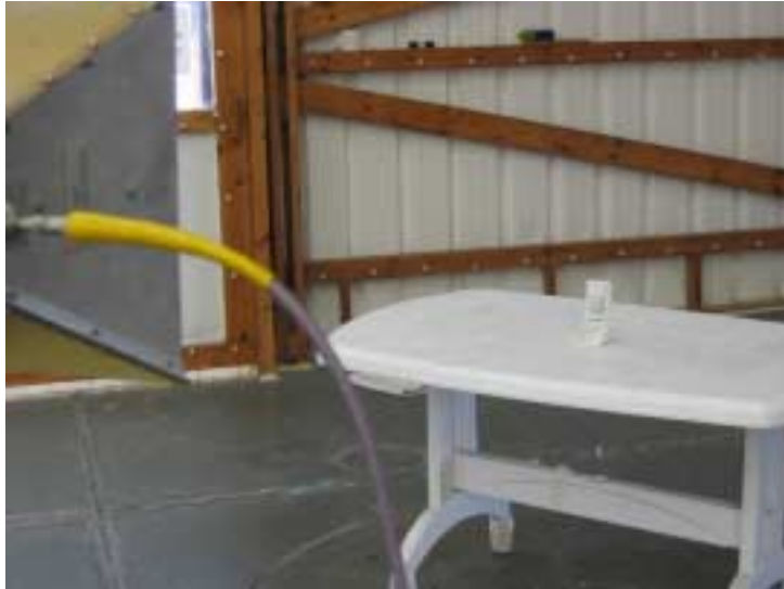
Photograph No.3 Setup for radiated emission measurements at the OATS from 1 to 18 GHz
