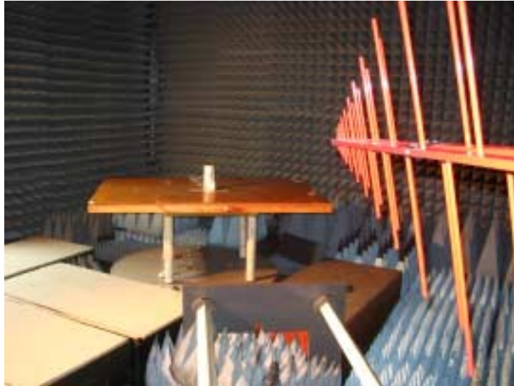
Photograph No.2 Setup for spurious emission field strength measurements in anechoic chamber in 30 MHz – 1000 MHz range
