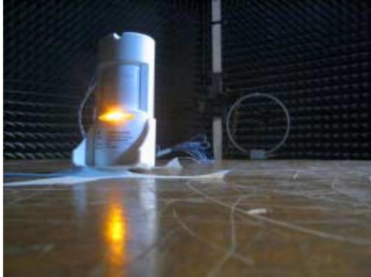
Photograph No.1 Setup for spurious emission field strength measurements in anechoic chamber below 30 MHz
