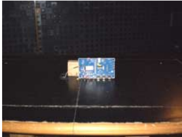
Photograph 7.4.3 Setup for spurious emission field strength measurements, close view
