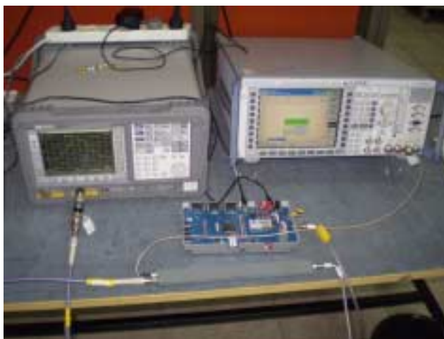
Photograph 7.1.2 Peak output power test setup
