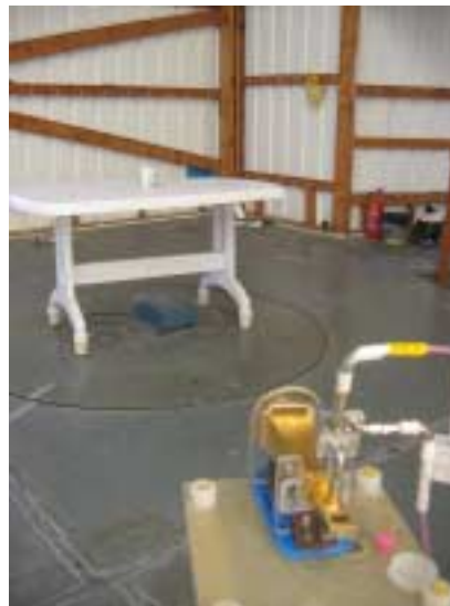
Photograph 7.1.6 Setup for spurious emission field strength measurements above 40 GHz
