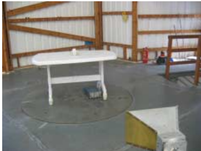
Photograph 7.2.1 Band edge emission measurement set up
