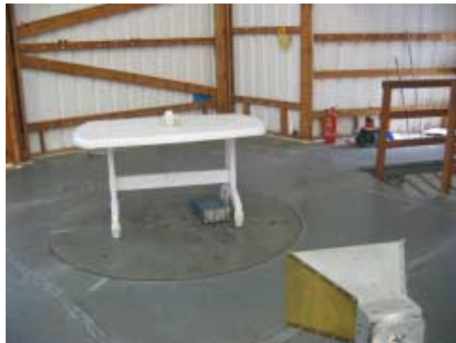
Photograph 7.1.3 Setup for spurious emission field strength measurements from 1 to 18 GHz
