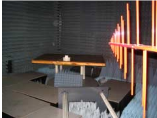
Photograph 7.1.3 Setup for spurious emission field strength measurements from 1 to 18 GHz
