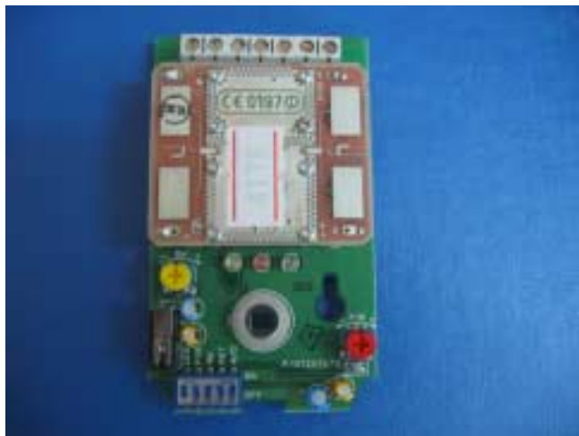
Photograph 8.2.3 Component side of the main PCB without RF PCB
