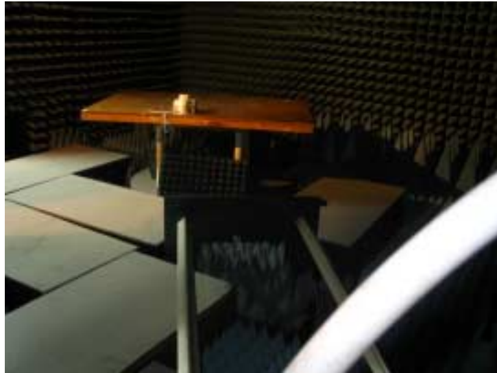
Figure 7.1.2 Setup for spurious emission field strength measurements above 30 MHz
