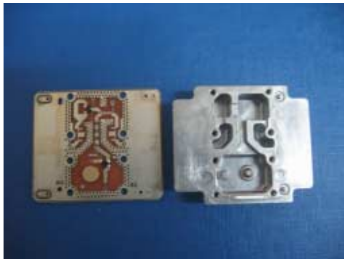
Photograph 8.2.7 Shielding compartments of the RF PCB
