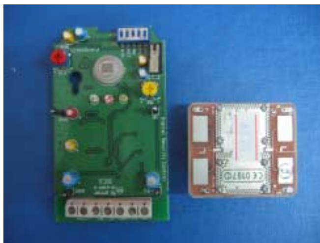
Photograph 8.2.3 Component side of the main PCB without RF PCB
