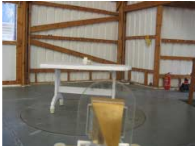
Photograph 7.1.5 Setup for spurious emission field strength measurements from 26.5 to 40 GHz
