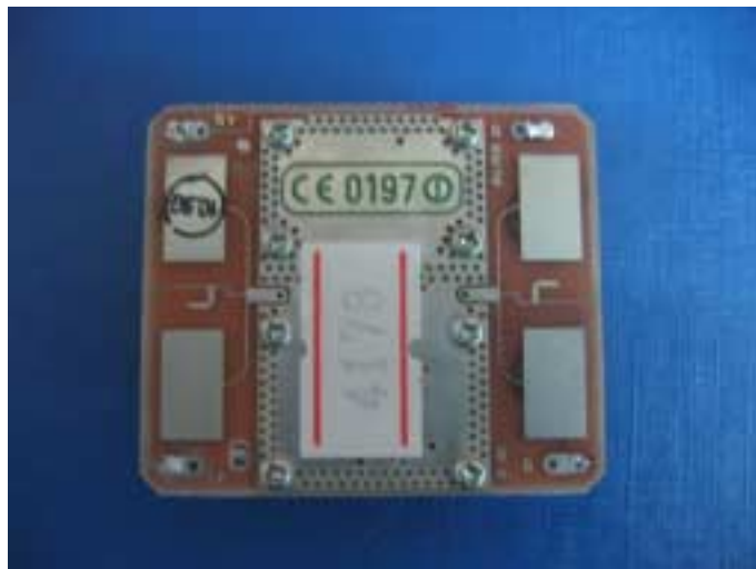
Photograph 8.2.7 Shielding compartments of the RF PCB
