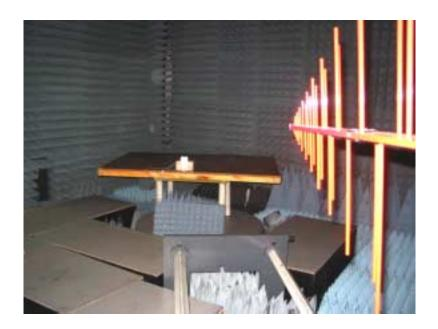
$\label{eq:Photograph No.3} \textbf{Setup for radiated emission measurements at the OATS from 1 to 18 GHz}$
