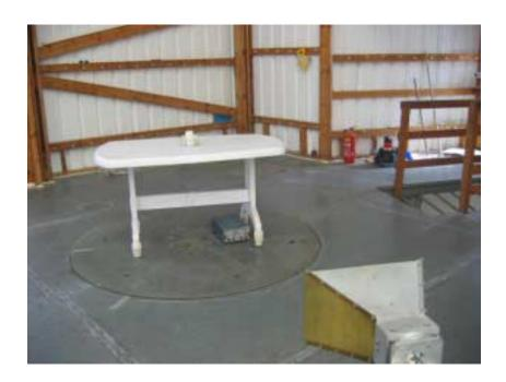
${\bf Photograph~No.4}\\ {\bf Setup~for~radiated~emission~measurements~at~the~OATS~from~18~to~26.5~GHz}$
