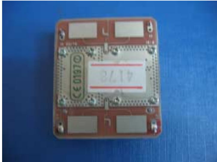
Photograph 8.2.6 Print side of the RF PCB
