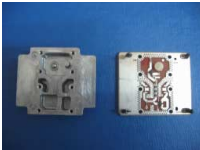
Photograph 8.2.7 Shielding compartments of the RF PCB
