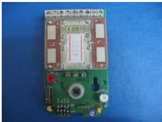
Photograph 8.2.2 Component side of the main PCB with RF PCB
