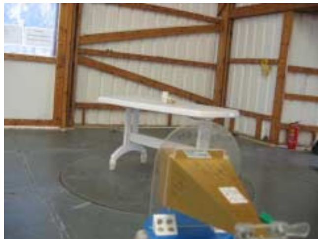
Photograph 7.1.4 Setup for spurious emission field strength measurements from 18 to 26.5 GHz
