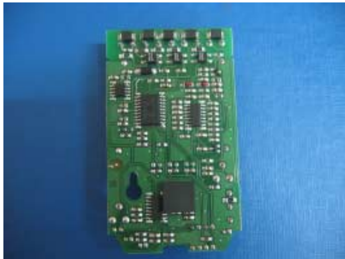
Photograph 8.2.4 Print side of the main PCB
