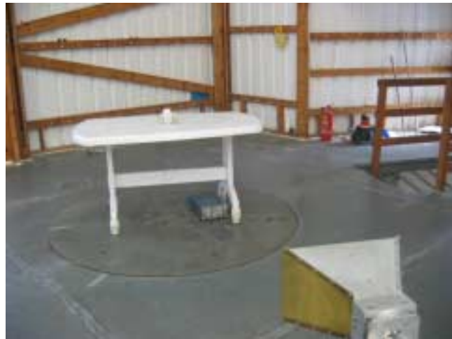
Photograph 7.1.4 Setup for spurious emission field strength measurements from 18 to 26.5 GHz
