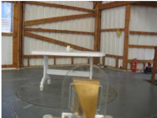
Photograph 7.1.6 Setup for spurious emission field strength measurements above 40 GHz
