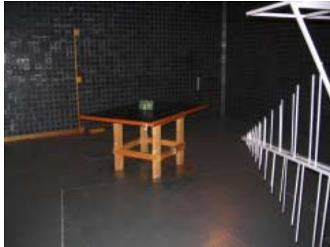
Photograph 9.2.1 Setup for radiated emission measurements, below 1 GHz
