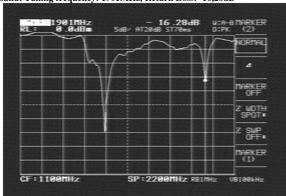
Fig 2. High band: Tuning frequency: 1901MHz, Return Loss: -16,28dB
