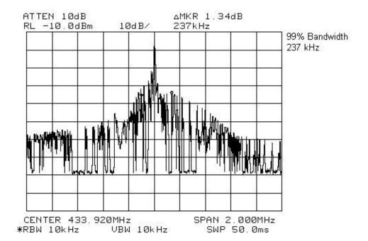
EQUIPMENT: Door Window Transmitter FCC ID F5303W4955
