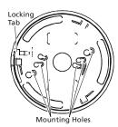
Secure backplate to the mounting surface using the screws provided. Note: Avoid mounting on uneven surfaces or electrical boxes. Warping of the backplate can result in a tamper.
