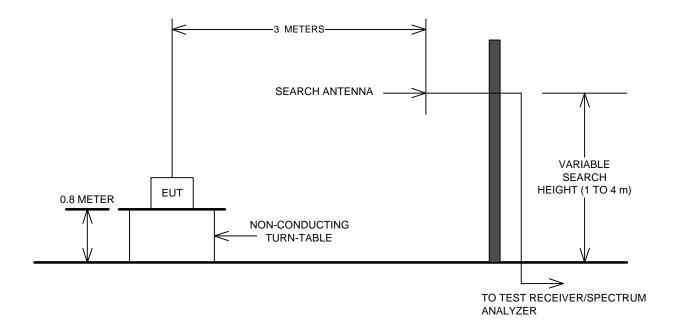
The spectrum was searched up to 1GHz or the 5<sup>th</sup> harmonic of the highest oscillator frequency, which ever was higher, up to a maximum of 40GHz.
