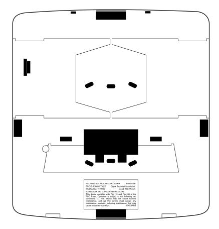
The FCC/IC labeling is to be located on the rear housing (08000XXX) of the unit as shown above. This illustration and labeling are shown 50% of the actual size.
