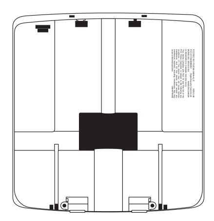
The FCC/IC labeling is to be located on the top of the rear housing (08000844) of the unit as shown above. This illustration and labeling are shown 50% of the actual size.
