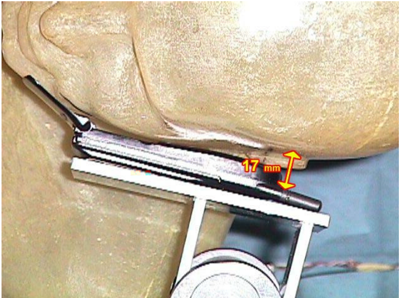
< Head Left Ear SAR Measurement – Close-up view >
