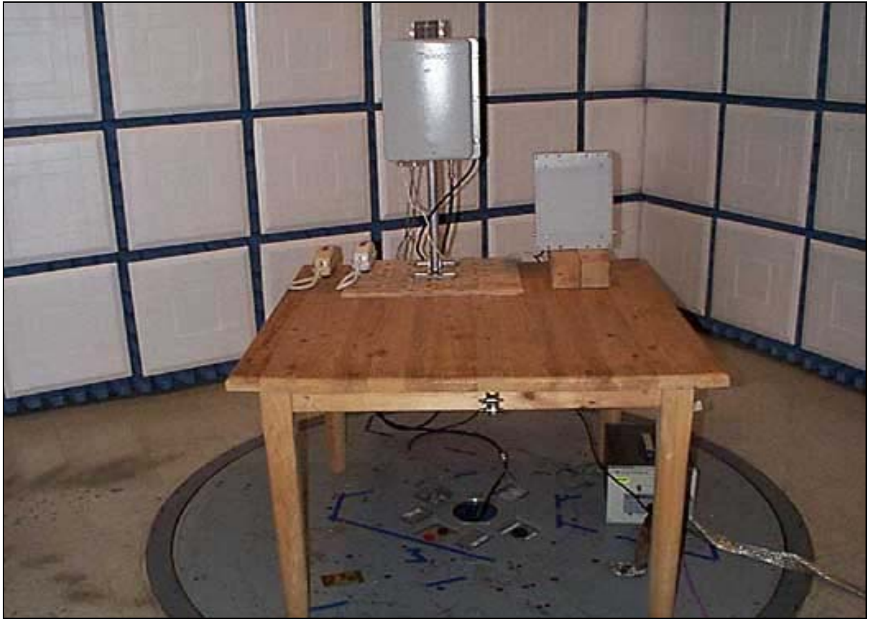
Mains Conducted Emissions - Front View
