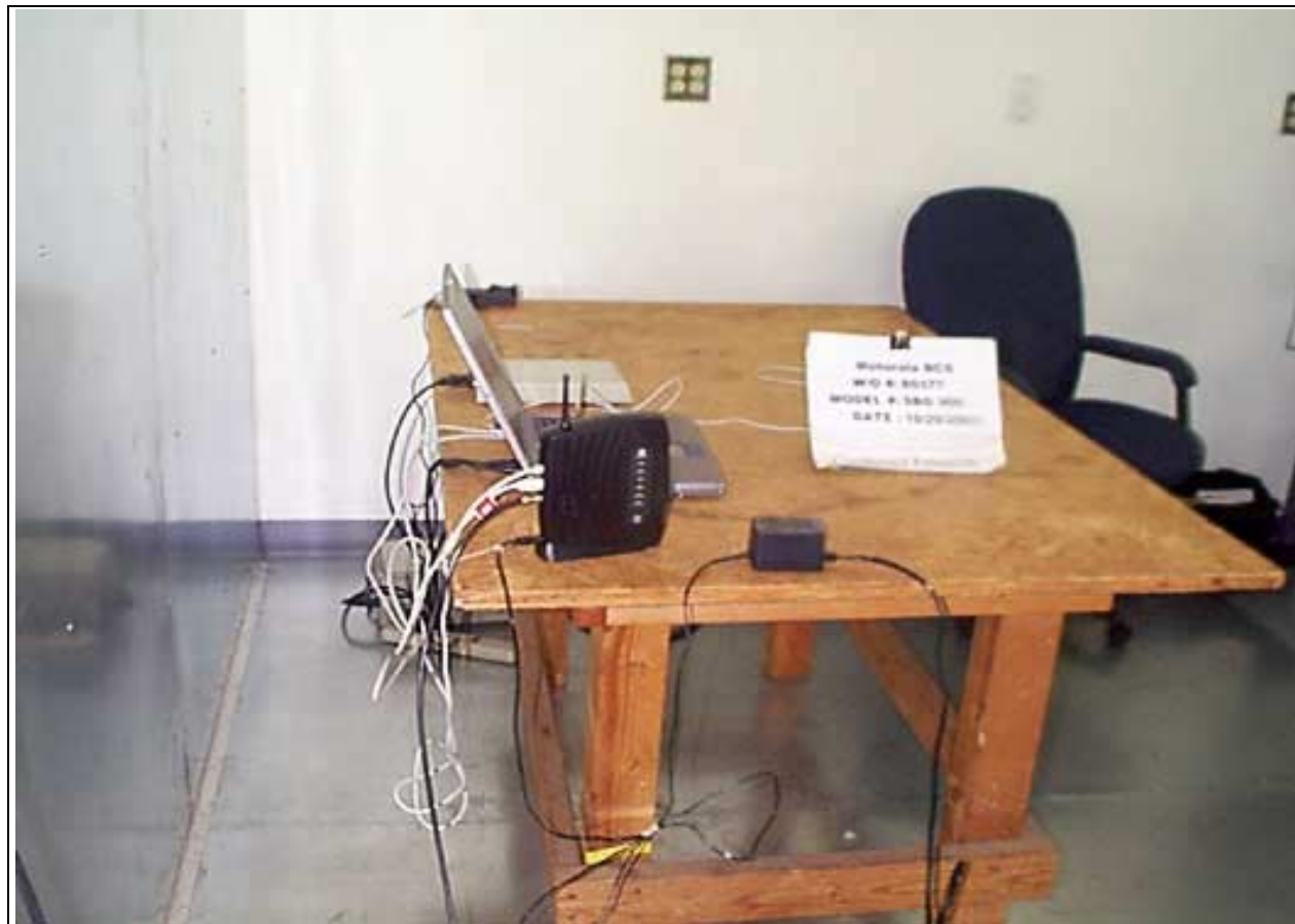
Mains Conducted Emissions - Side View
