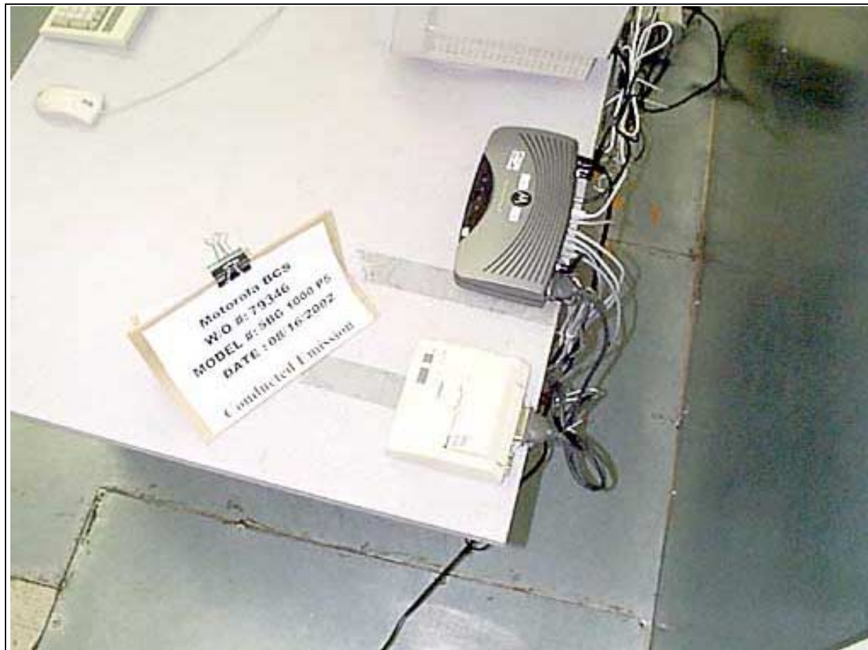
Mains Conducted Emissions - Back View
