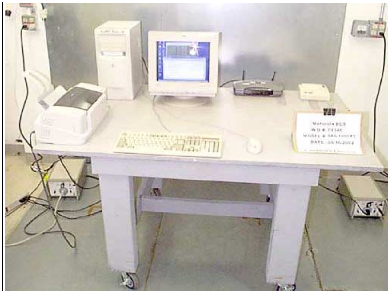
Mains Conducted Emissions - Front View
