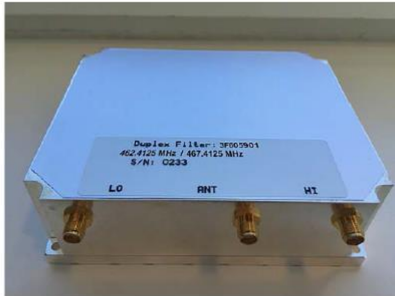
3F605901 – Duplex Filter Front
