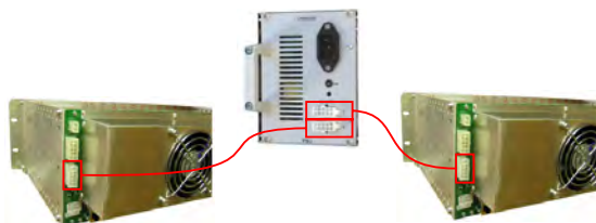
Backup Power for Two Master Units
