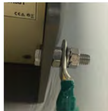
Figure 49 Remote Ground Connection
