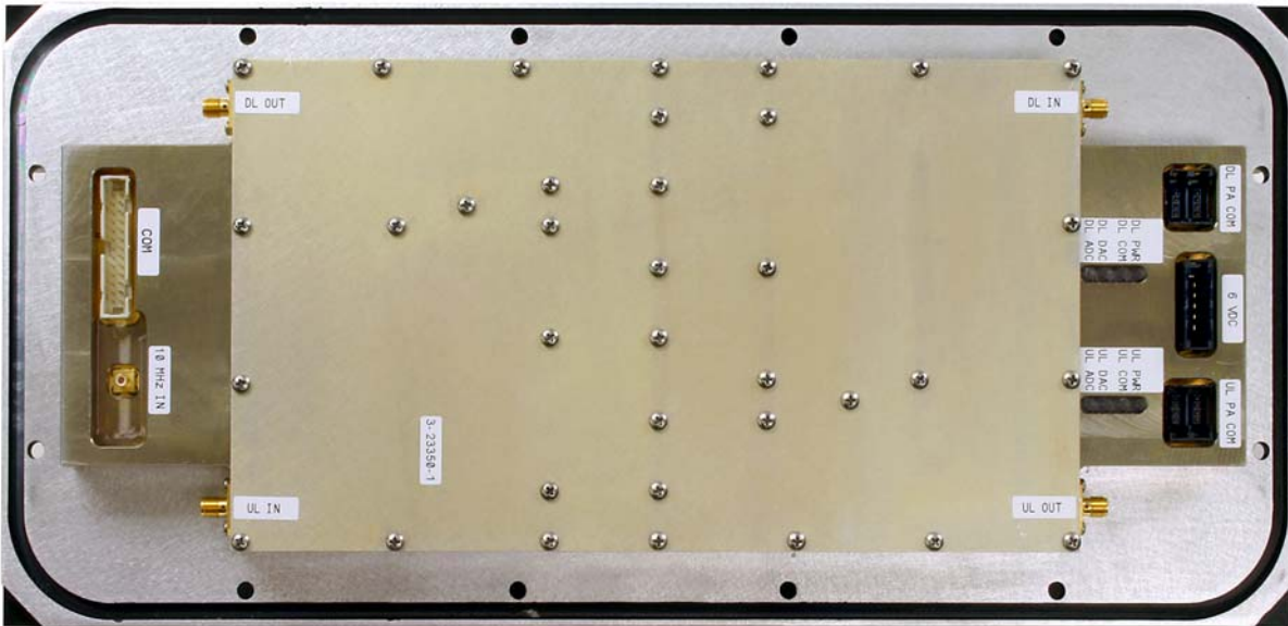
Channel Module 3-23350-1, 3-23368-1, 3-23919, 3-23920, 3-23921, 3-23922, 3-23923, 3-23924 top view (3-23350 shown as example, all modules have same physical appearance except for the part number sticker).
