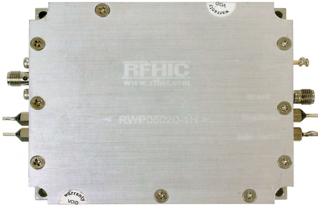
Power Amplifier 8-23291 top view.
