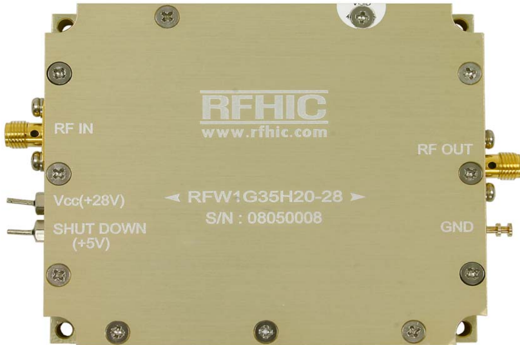
Power Amplifier 8-22290 top view.
