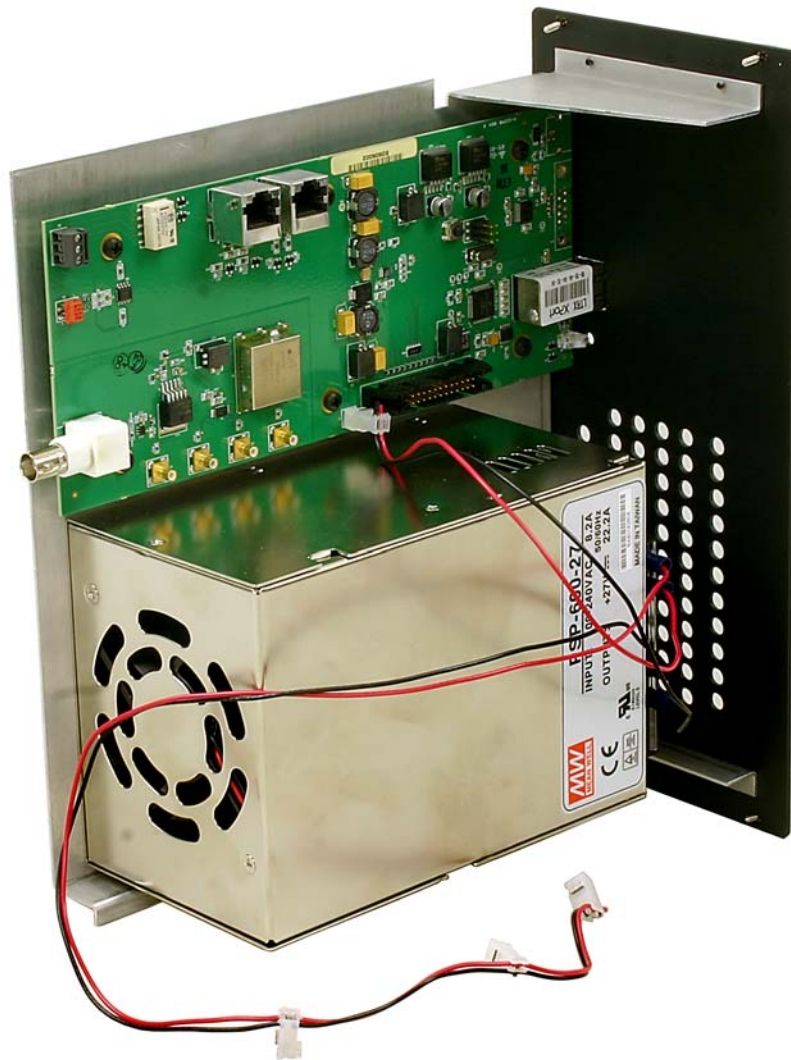
Power Supply (8-22688) and Control Board (3-22299).
