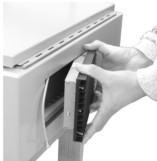
Figure 11: Slide amplifier towards bottom of cabinet to remove upper cable.
