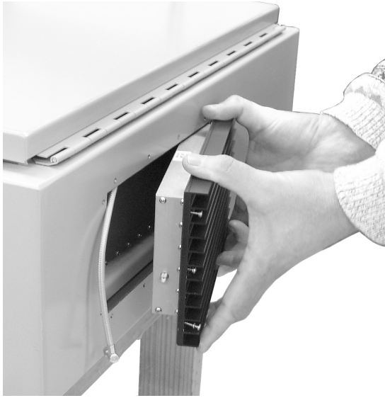
Figure 12: Slide amplifier towards bottom of cabinet to remove upper cable.
