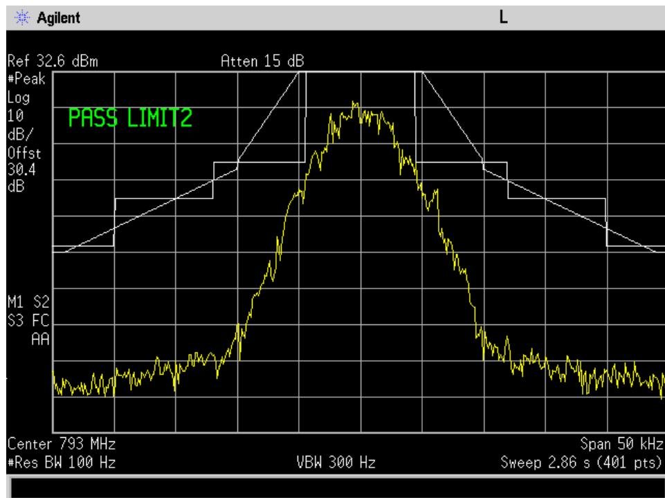
**Uplink low ch Mask C and B\_+3dB**
