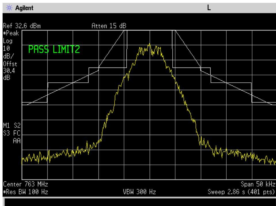
**Downlink low ch Mask C and B\_+3dB**
