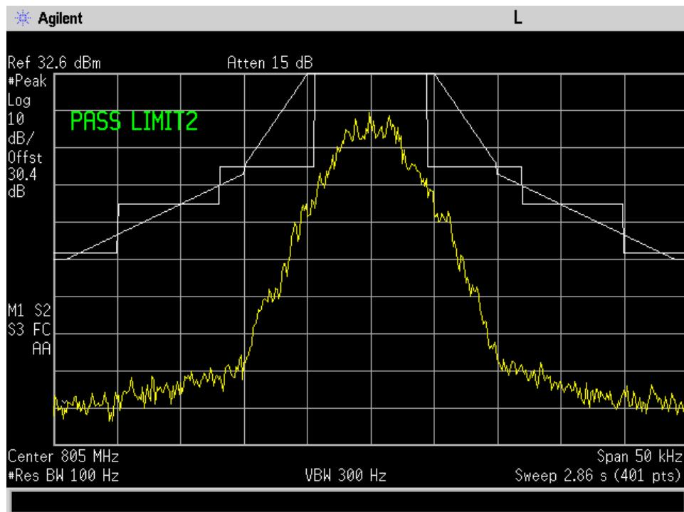
**Uplink high ch Mask C and B\_+3dB**
