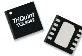
10-pin 3 x 3 mm DFN Package
