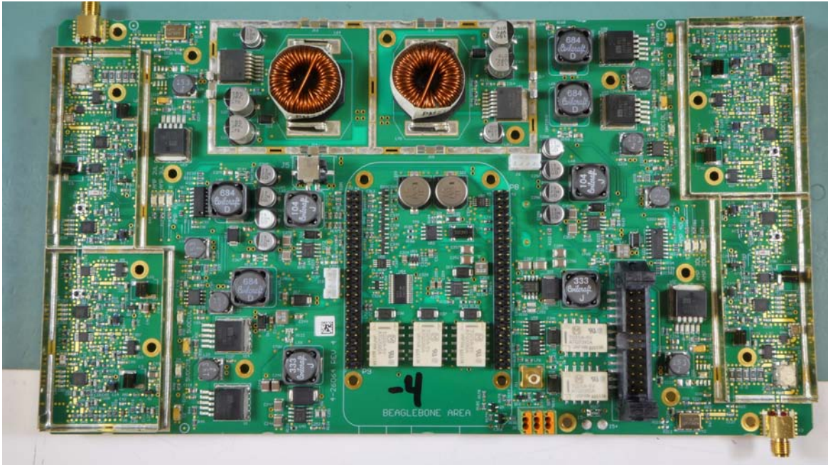
Control and LNA PCBA 3-26063-4 Front view
