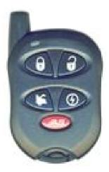
N.B.: Pressing the Aux then LOCK button will activate the Aux 2 output.
