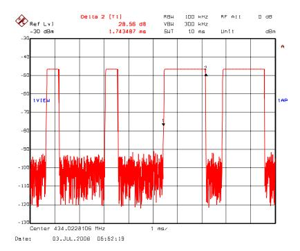
**Duty Cycle in 100ms:**  $(28 \times 1.74 \text{ms}) + (12 \times 541.08 \text{us}) = 48.72 \text{ms} + 6.49 \text{ms} = 55.21 \text{ms}$ **Duty Cycle Factor** =  $20 \times (0.5521) = -5.16 \text{dB}$
