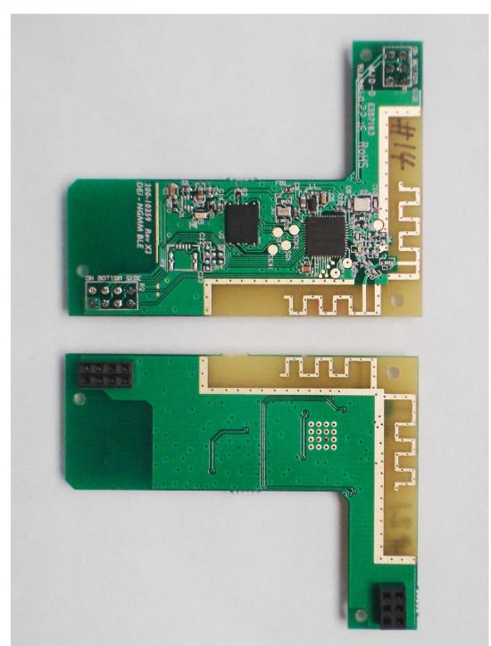
This is the photo of prototype Rev X2, submitted for the FCC Certifications test. The Rev 3.0 is identical in every aspect, with the printed information FCC ID: EZSDEIBLE1 and IC:1513A-DEIBLE1.
