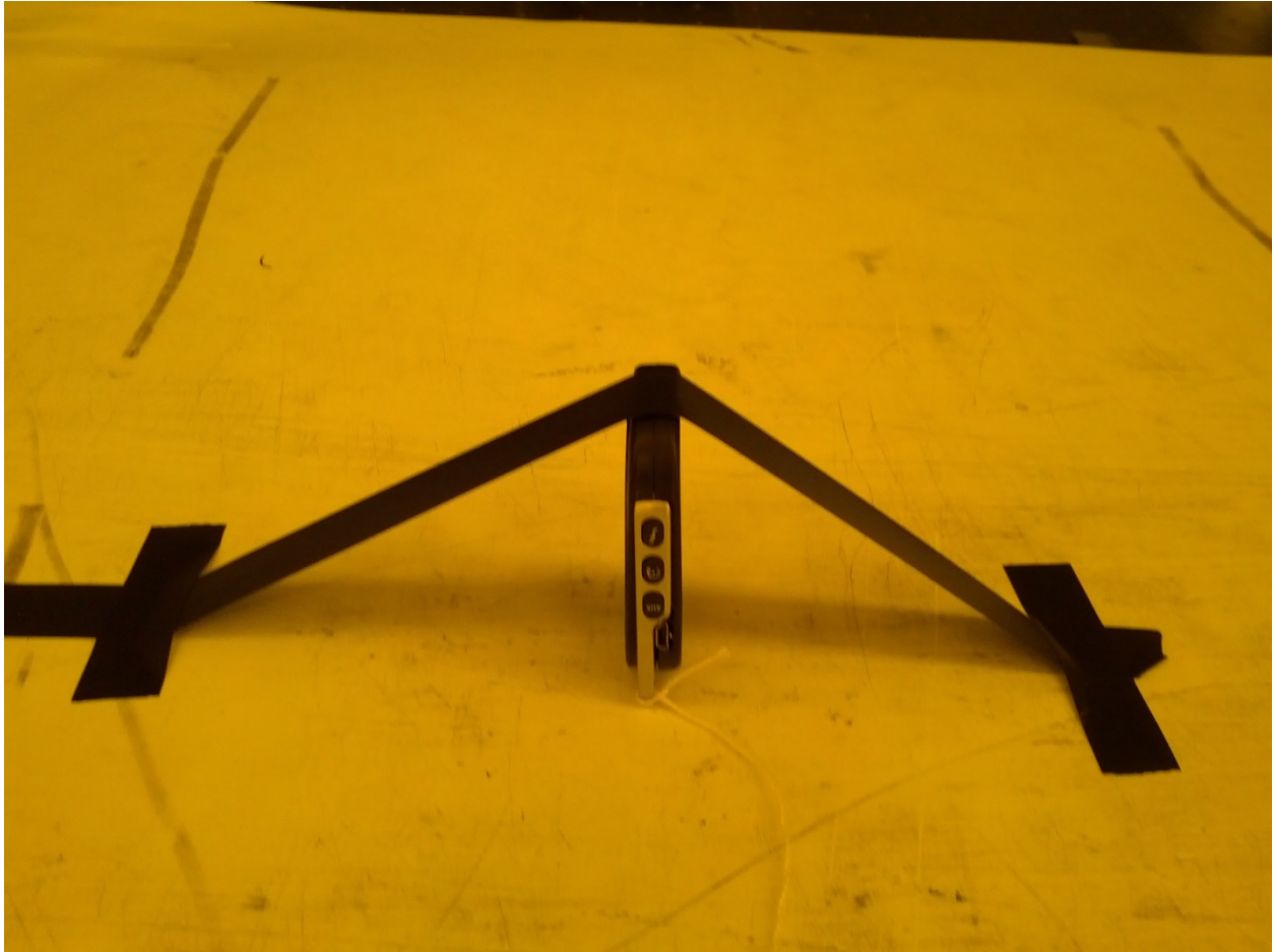
Photograph 4 – EUT Orientation for Radiated Tests - Vertical
