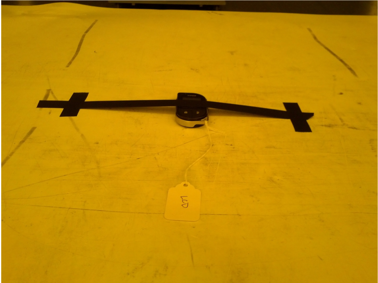
Photograph 3 – EUT Orientation for Radiated Tests - Flat
