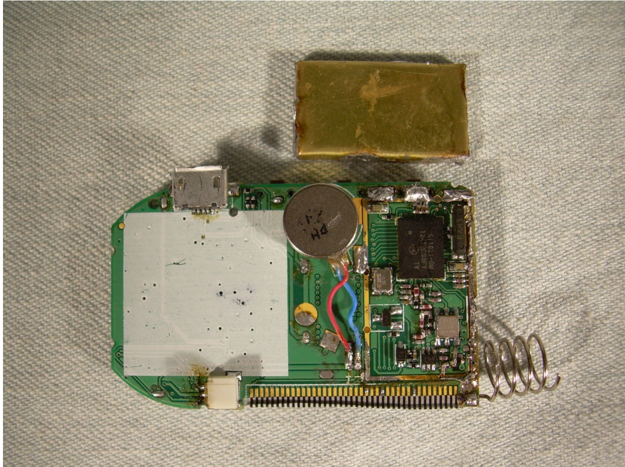
Photograph 7 – View of the Back Side of the PCB with RF Shield Removed
