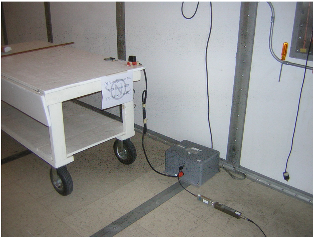
AC power line conducted emissions, MODEL 6703A, no enclosure
