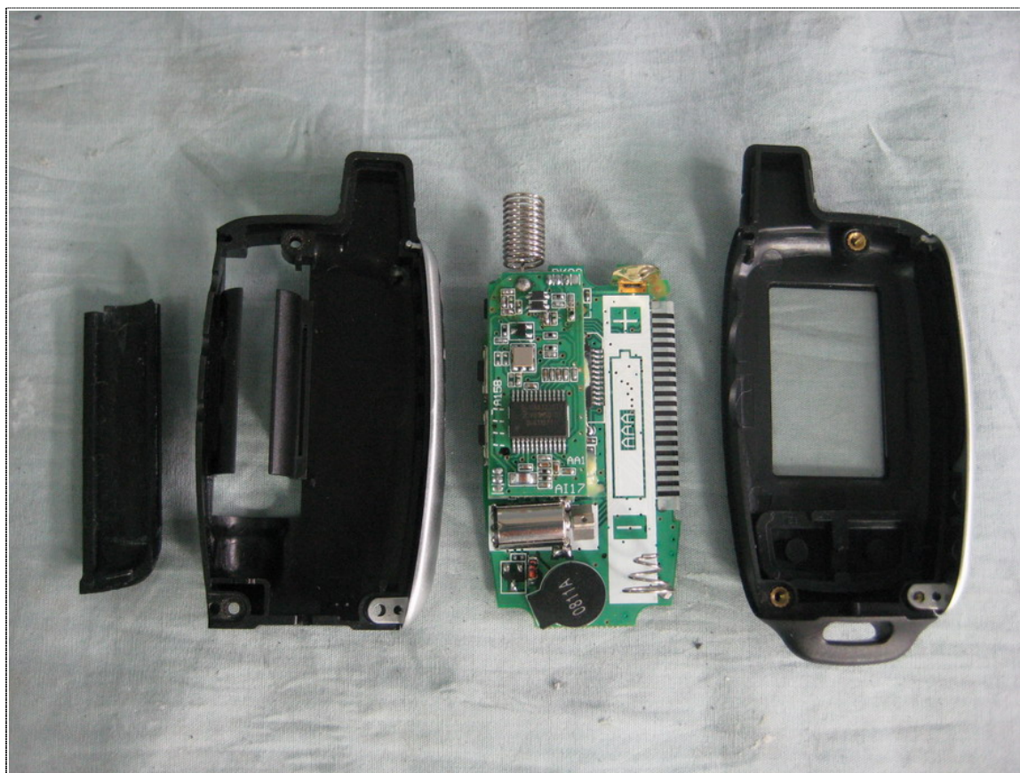
Inner View of EUT
