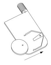
3. With the front and circuit board still turned over, turn back portion of unit onto both parts, reposition all parts and snap together.
