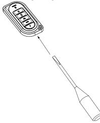
1. Using a small flathead screwdriver, insert into slot located at the bottom of the keypad and carefully pry the front of the unit open.
