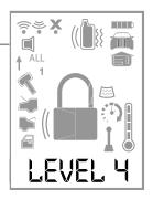
The alarm arms, doors lock, and the siren chirps and parking lights flash 4 times. The **FULL SILENT ARM** text and beeps play to confirm and the system and siren icons update.
