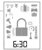
The alarm arms, doors lock (if connected), and the siren chirps and parking lights flash once. The **ARMED** text and beeps play to confirm and the system status icons update. If valet mode\* is on, the doors lock and the **VALET** text and tone play. Exit valet mode to arm the alarm normally.
