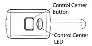
The control center, typically located on the upper part of the front windshield sends and receives commands or messages to and from your system. It consists of:
