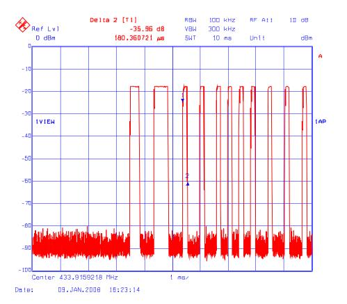
**Duty Cycle in 100ms:** (1 x 380.76us)+(1 x 541.08us)+(57 x 180.36us)= 0.381+ 0.541 + 10.281ms= 11.20ms **Duty Cycle Factor** = 20\*log(0.1120)= -19.02dB
