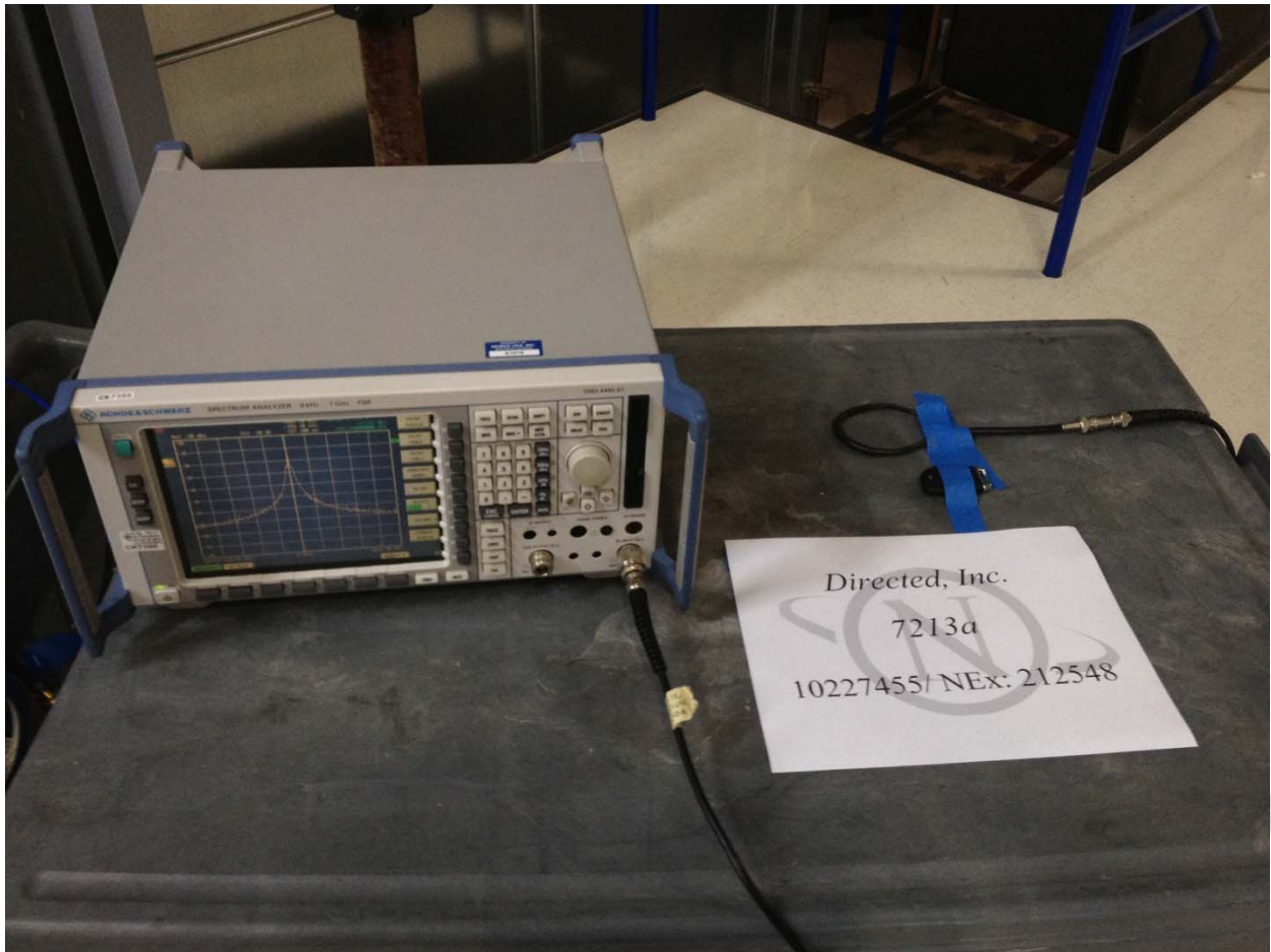
Occupied Bandwidth Test Setup
