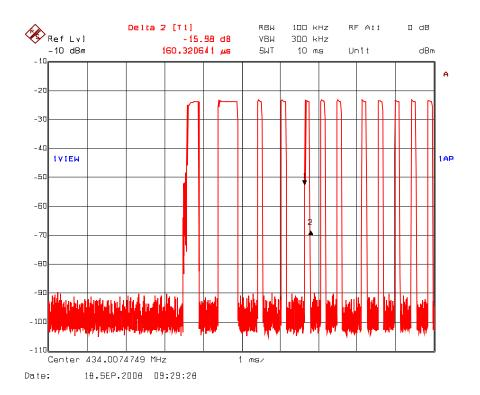
**Duty Cycle in 100ms:** (1x340.7us) + (1x521.0us) + (57x160.32us) = 10ms**Duty Cycle Factor** = 20\*log(0.1) = -20 dB
