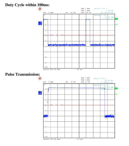
Due to FSK modulation Duty cycle within 1 pulse is 100%.
