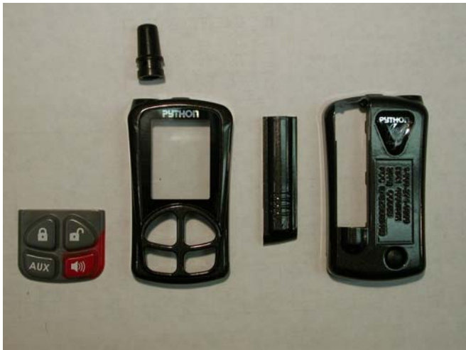
Photo 9 Exploded view of plastic case assembly
