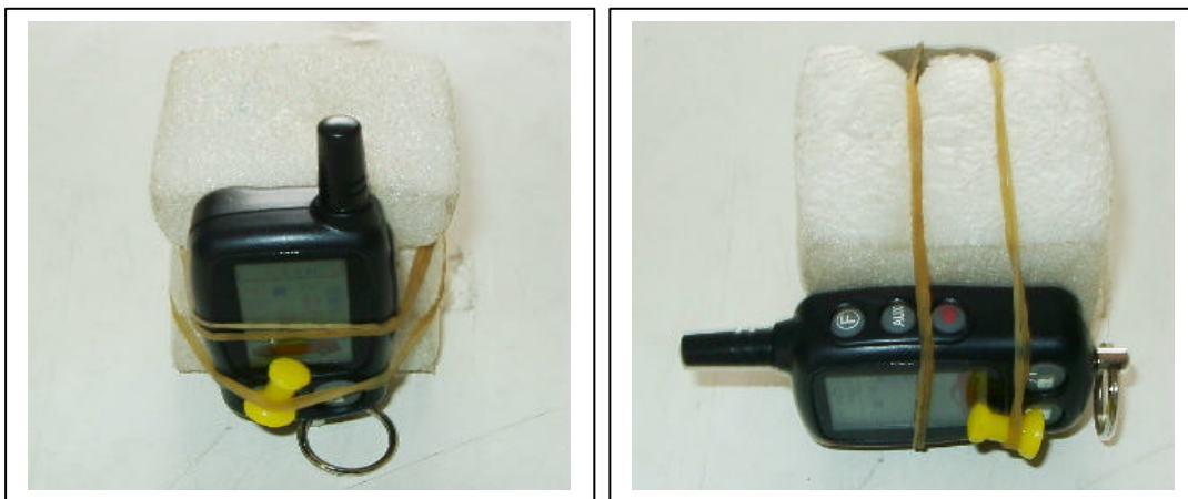
Radiated Open Site Test Set-up (Transmitter Mode)
