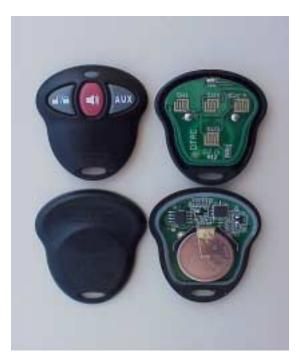
**Photo 2** Original 4 button configuration. Again, same PCB is used for either 3 or 4 button configuration.
