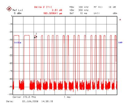
**Duty Cycle in 100ms:**  $(2 \times 521.04 \text{ us})+(57 \times 160.33 \text{ us})=1.04208 + 9.13881 \text{ ms}=10.18089 \text{ ms}$  **Duty Cycle Factor** =  $20 \log(0.1018089)=-19.84 \text{ dB}$
