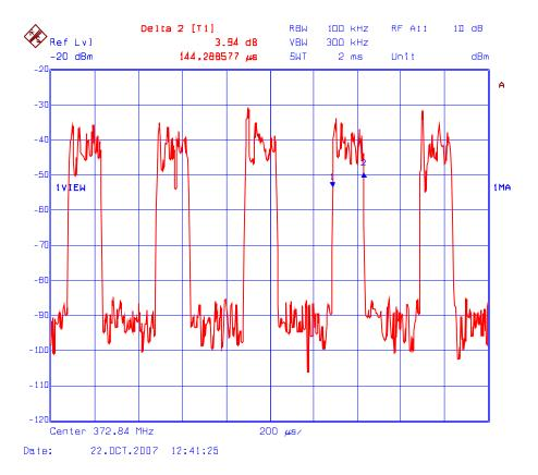
**Duty Cycle in 100ms:**  $(61 \times 144.2885 \text{us}) = 8801.59 \text{us} = 8.8016 \text{ms}$  or 8.8016 % in 100ms **Duty Cycle Factor** =  $20*\log(0.088) = -21.11 \text{dB}$
