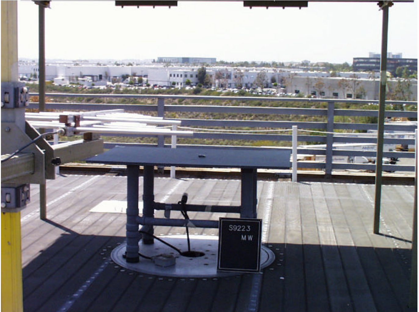
Photograph of Test Setup: Radiated Emissions 30 MHz - 3.144 GHz
