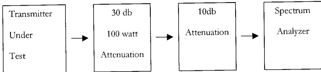
**TRANSMITTER POWER MEASURED IN dbm***[Refer to Sections 2.985 and 2.991]*
