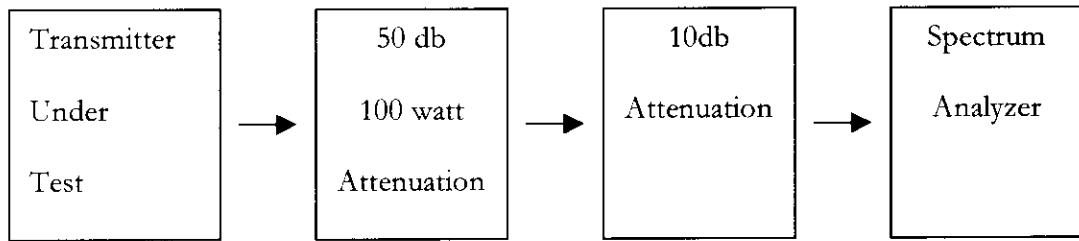
**TRANSMITTER POWER MEASURED IN dbm***[Refer to Section 2.991]**(Table 6.2)*
